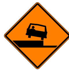
TC-49 PAVEMENT DROP-OFF
