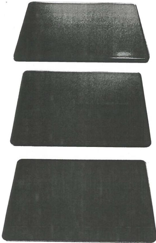
EXAMPLE METAL WITH PROPOSED IRIDESCENT FINISH 3 SAMPLE PHASES SHOWN [BOTTOM TO TOP: ALL GREEN, PARTIAL GREEN/COPPER, ALL COPPER] VISIBLE COLOUR SPECTRUM WILL DEPEND ON ANGLE OF SIGHT TO MATERIAL, AVAILABLE LIGHT / SHADOW, ETC.
