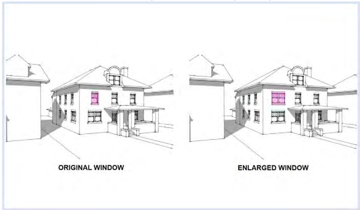
Figure 31: The illustration shows an enlarged window on a heritage building.
