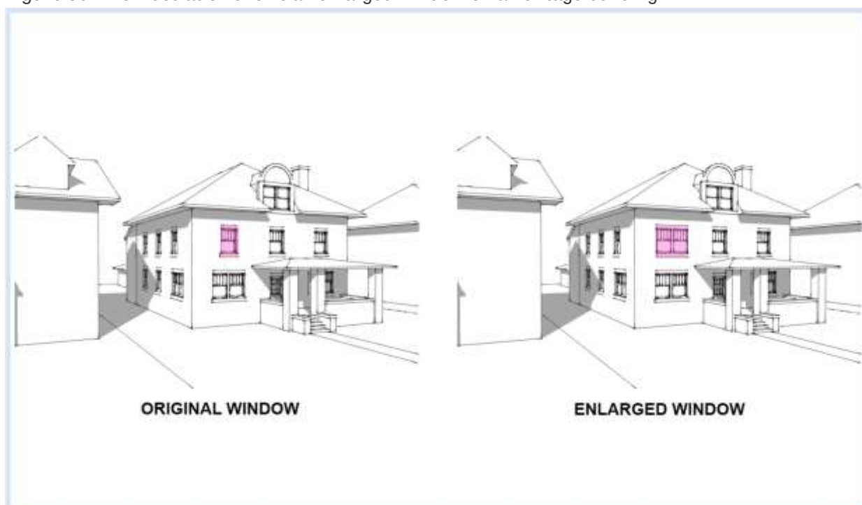
Figure 30: The illustration shows an enlarged window on a heritage building.
