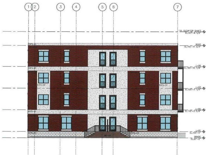
EXTERIOR ELEVATION - WEST 1/8" = 1'-0"
