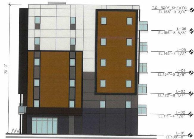
2 EXTERIOR BUILDING ELEVATION - SOUTH SK-04 1/16" = 1'-0"
