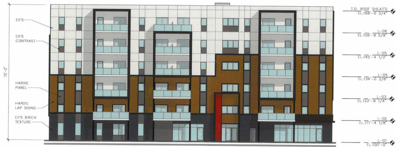
1 SK-03 EXTERIOR BUILDING ELEVATION - WEST 1/16" = 1'-0"
