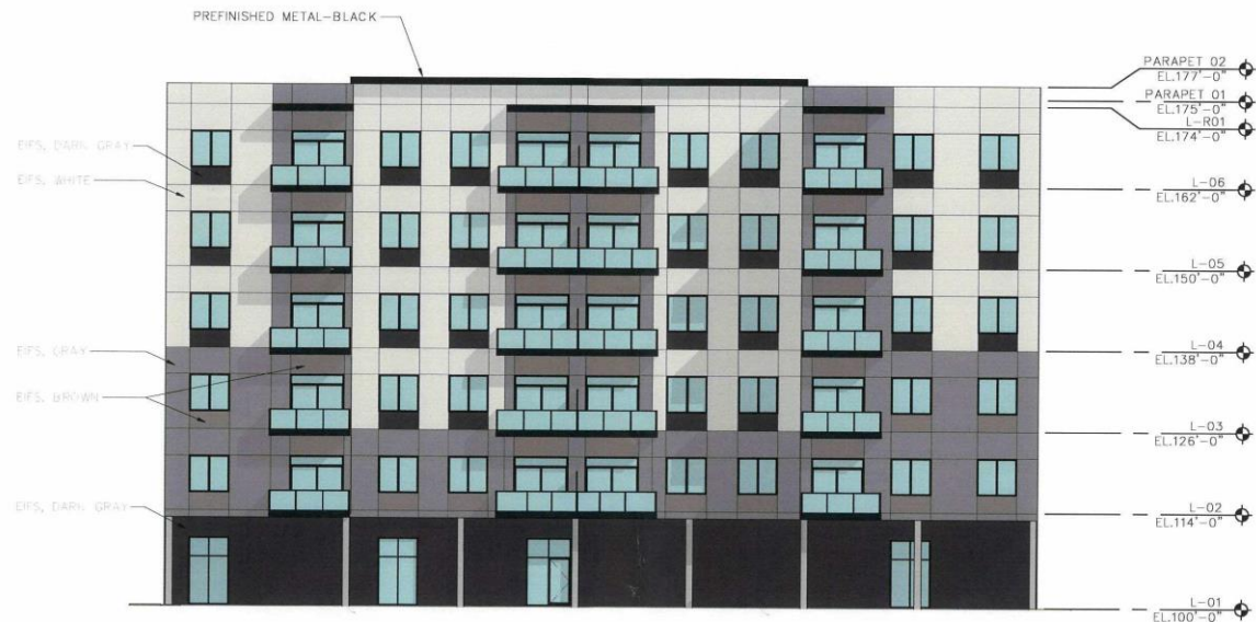
1 SK-08 BUILDING ELEVATION - NORTH 1/16" = 1'-0"
