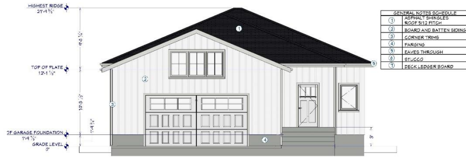
E1 EXTERIOR ELEVATION FRONT 1/8 IN = 1 FT
