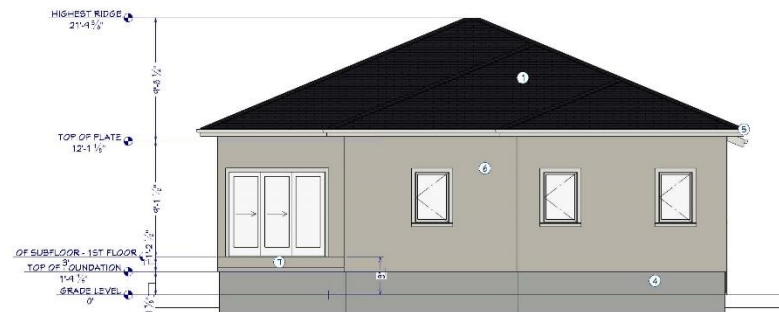
E3 EXTERIOR ELEVATION BACK 1/8 IN = 1 FT
