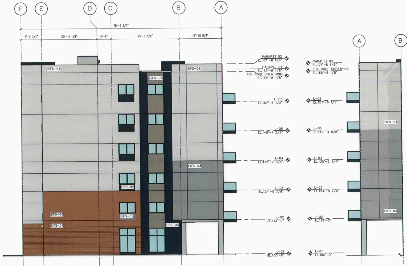
2 BUILDING ELEVATION - EAST A4.2 1" = 10'-0"
