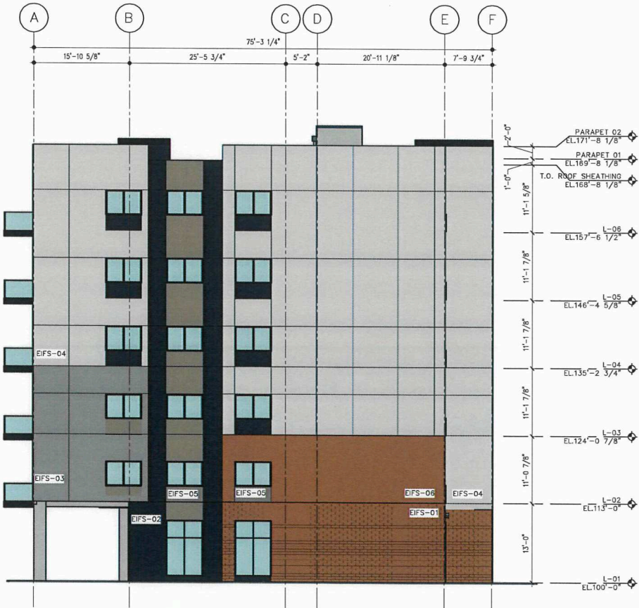
2 A4.1 BUILDING ELEVATION - WEST 1" = 10'-0"
